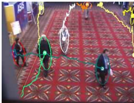
Video Analytics software tracks people and objects, and can send alarms when suspicious activities occur.
